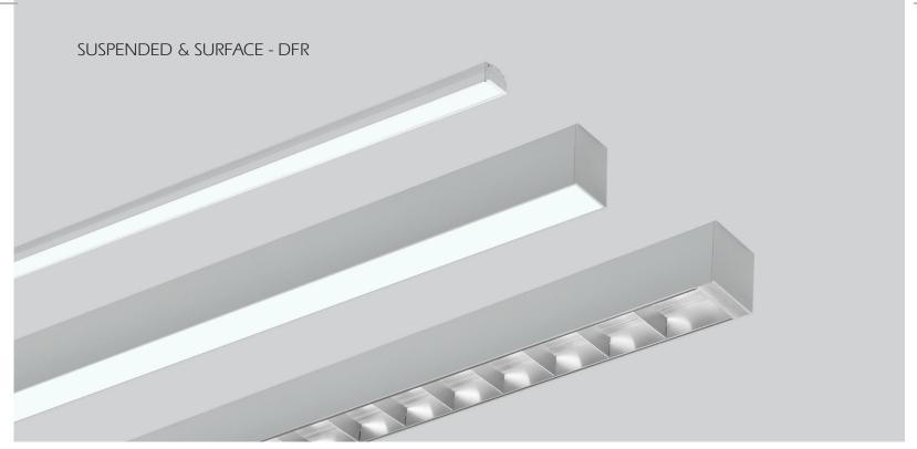
EOSLED luminaries, which can be used as surface-mounted or pendant, are produced with the widths of 20 - 60 - 80 mm. They can be used as a single profile with the length of up to about 2,5 m in linear applications. It is possible for it to be used as a light source by attaching from end to end. Thanks to special mounting apparatuses, pendant length can easily be adjusted.
