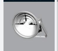
Body, cover and frame in die-cast aluminum, painted in gray color. Tempered glass pressed on silicone gasket. Internal reflector/baffle in aluminum and steel to cut down the upward light output keeping unchanged the flux of the aiming direction. Fixing bracket in galvanised steel with aiming goniometer in die-cast aluminum painted in gray.
