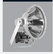
Body, in die-cast aluminum painted in gray color. Tempered glass pressed on silicone gasket. Safety insulator block for maintenance block for maintenance operations when opening the cover. Turned reflectors in matt finishing. Fixing bracket in galvanised steel with aiming goniometer in die-cast aluminum painted in gray.
