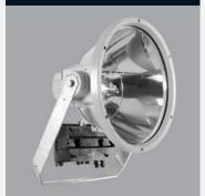
Body, in die-cast aluminum painted in gray color. Tempered glass pressed on silicone gasket. Safety insulator block for maintenance operations when opening the cover. Turned reflectors in brightened specular aluminum. Fixing bracket in galvanised steel with aiming goniometer in die-cast aluminum painted in gray.
