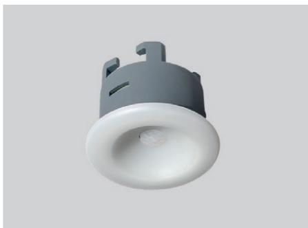
Multi sensor is implemented in the biodynamic lighting solution in order to maximise efficiency. The multisensor receives user settings from the touchpad and transmit these as well as occupancy and daylight lux data to the controllers on the network.
